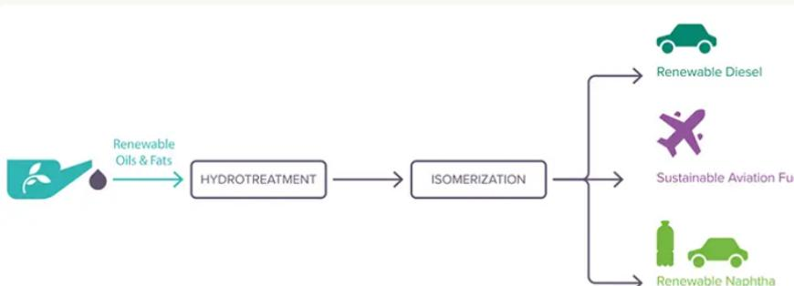
According to Axens, its "Vegan" technology is a second-generation hydrotreated vegetable oil (HVO) solution that processes up to 100 percent of any kind of lipid, including wastes from agriculture and the food industry to produce renewable fuels that are able to reduce greenhouse gas (GHG) emissions by up to 80 percent compared with a conventional jet fuel production scheme (graphic courtesy Axens).
